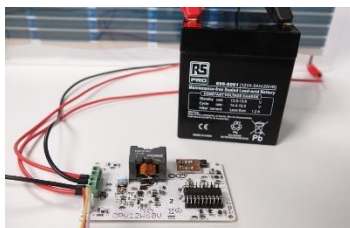
OPV12W60V connected to SOLO panel and battery
